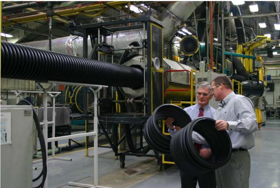
FINDLAY, Ohio - During his tour of the ADS plant here, Congressman Robert Latta (R-Ohio) (left) examined a sample section of corrugated high-density polyethylene (HDPE) pipe. ADS Findlay, Ohio Plant Manager Steve Farrow explained how the pipe is designed and made to be strong, and that even standard 20-foot sections can be installed by a crew with minimal equipment. (Photo by ADS)
